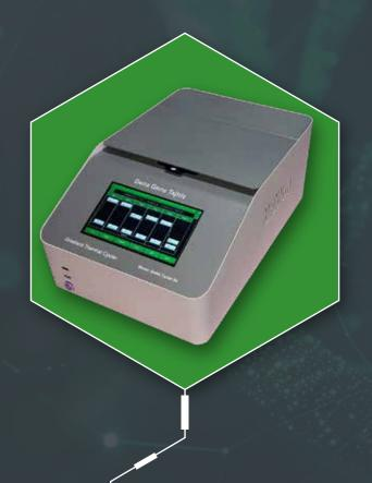
The thermal cycler, or PCR machine, utilizes Peltier technology to amplify nucleic acids. By amplifying DNA, subsequent downstream processes such as diagnostics, cloning, genotyping, and sequencing can be easily performed.
