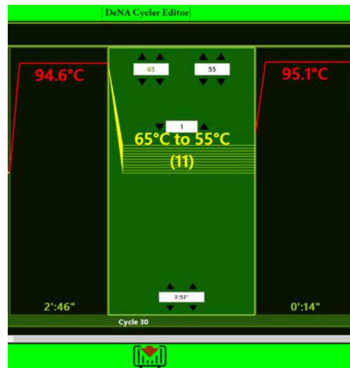
Figure 16. Touch Step Settings. The Touch Step can be either Touch Down or Touch Up.
