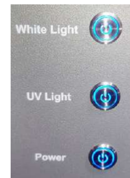
Figure 1. Gel Documentation Panel Buttons. Note that the illumination of the button lights does not indicate that the corresponding option is activated. The user must press the respective button downward to enable the desired function.
