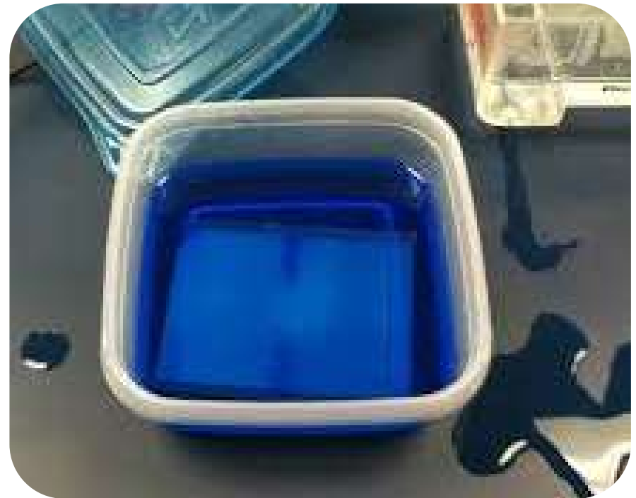
Figure 3. Staining Bath for Protein Staining in Acrylamide Gel
