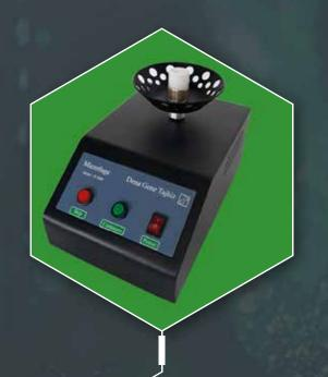
The microcentrifuge vortex mixer (Spin-Vortex) is a simple laboratory device that can perform vortexing, mixing, centrifugation, and sample separation operations. Its primary application is in cellular and molecular laboratories. This device is most commonly used in the spin-down of PCR products and mixing of PCR reactions.
