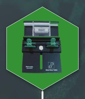
The gel casting system is used to facilitate the agarose gel preparation process as an auxiliary device for horizontal electrophoresis. Initially, it is necessary to place the blocking movable piece and then the threaded movable piece onto the base piece.
